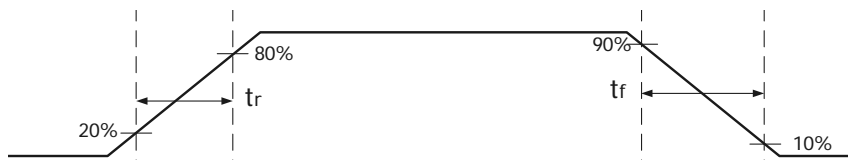
Figure 2. Definition of Rise Time and Fall Time
